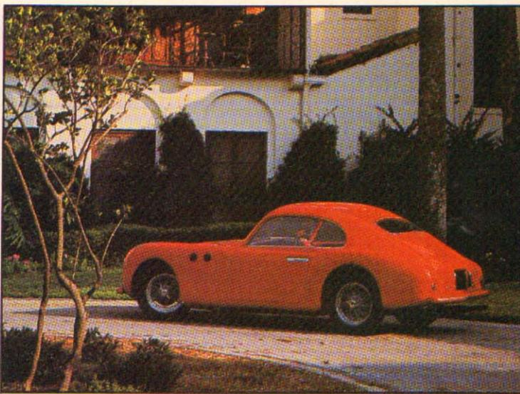
the roof tapered inward as well as downward to a very small Kamm tail. The underside of the car was as carefully studied as the upper; favorable airflow tests in the Politecnico di Torino *galleria del vento* were confirmed by a speed of 201 km/h (a whisker under 125 mph) actually achieved by the car, 202 CMM number 001, on the Torino-Milano *autostrada* in April 1947. It should be emphasized that this speed was reached with a 1089-cc, 4-cylinder engine producing only 61 bhp.
